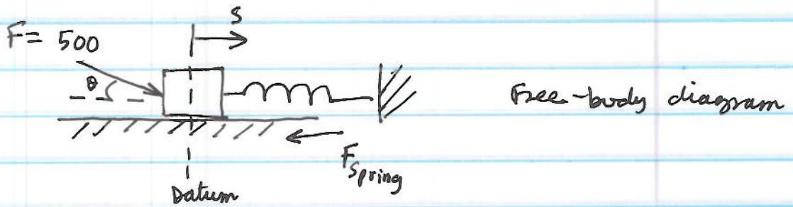
so the applied force causes the motion which in turn compresses the spring. So the work of this force causes energy to be stored in the spring.
