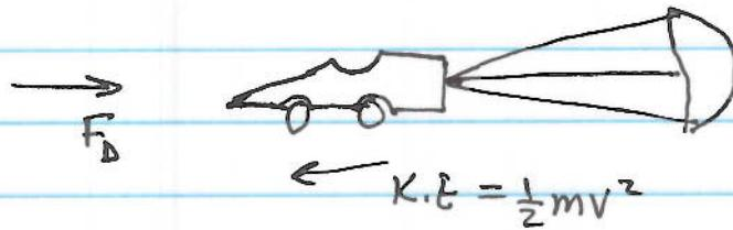
Once ~~breaks~~ engine is shut off dragster moves by its inertia and only force acting on it is the drag force  $F_D$ .
