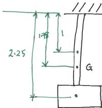
So this is a composite, so the MMI is the algebraic sum of the MMI of the components. We can find MMI of each component about its center of mass, then use the Parallel Axis Theorem to convert it to MMI about center of mass of the system  $G$ ,
